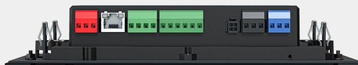
Power In PoE Ethernet 2x Digital Out 5x Digital In USB 2.0 Host 2x Add-On Port
